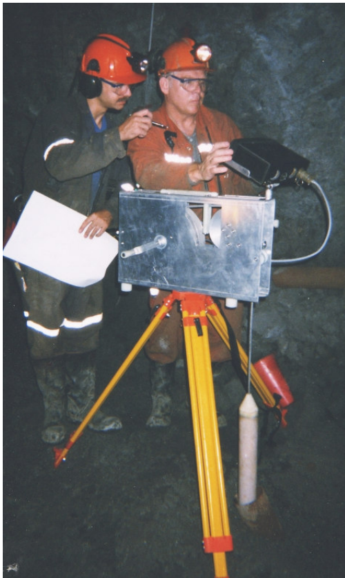
A Falconbridge crew (Steve Falconer and Chris Morley) logging production holes with the GDD SSW system at Craig Mine, Sudbury.
