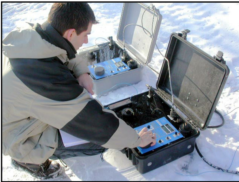
Model TxII in Master/Slave mode providing up to 7,200W-4800V-15A
