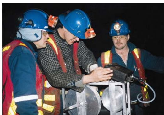
Rysunek 4: Ron Lemery, Ken Germain and Mario Fluet at Raglan Mine are setting the SSW system to verify ore contacts in their blast holes
